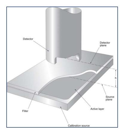
Figure 1: Definition of source-detector positioning
