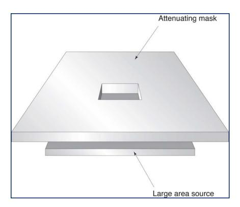
Figure 3: The use of a mask to simulate a small area source
